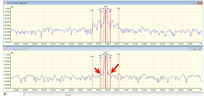
Figure 6: Peaks associated with bearing conditions with the red arrows showing the outer race frequencies in voltage spectra.
