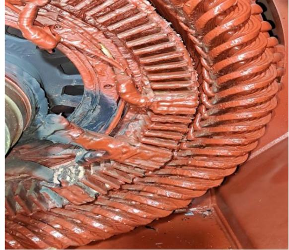
Figure 2: Failed rotor connection and wye ring failure detected early.
