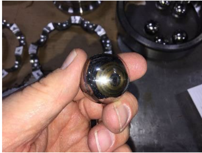
Figure 6: Bearing ball damage from the ground currents in Figure 5.
