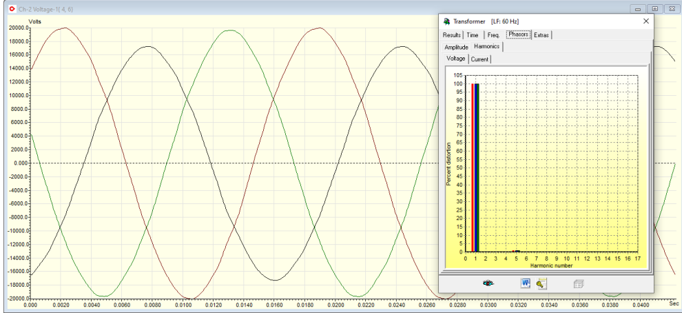
Figure 1: Relatively clean voltage waveform with less than 1% THD voltage.
