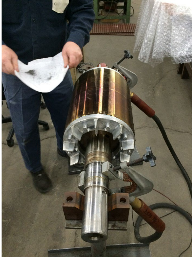
Figure 10: Induction rotor undergoing rotor 'growler' testing following overheating of the rotor (discoloration) from high power and ground harmonics.
