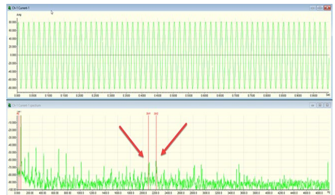
Fig. 4. Wedge signature in an 800 hp induction motor
