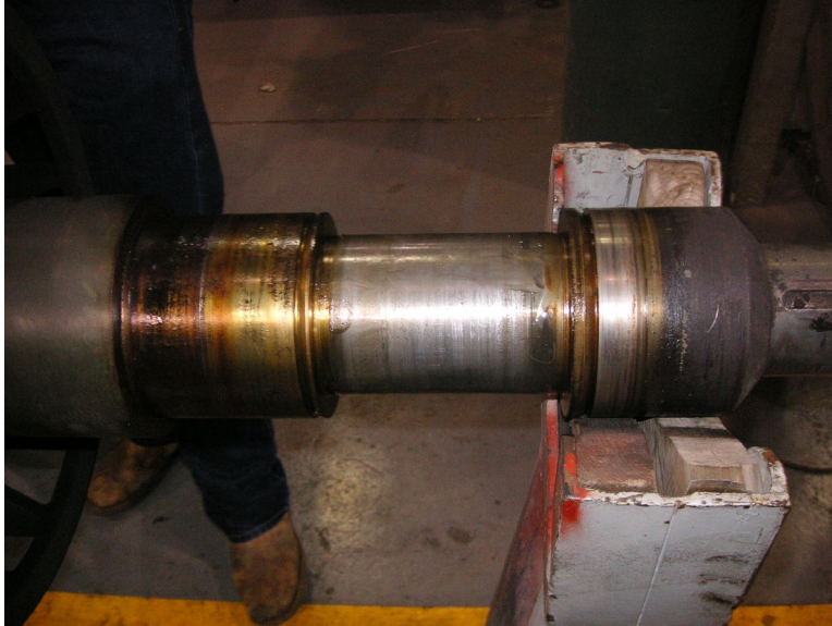
Figure 11: Failed Seal Surface on the Rotor
