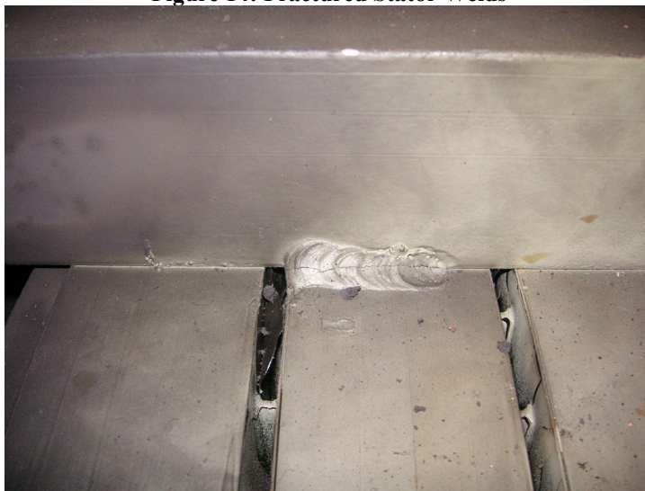
Figure 14: Fractured Stator Welds
