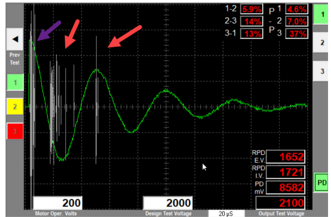
Fig. 4. Example of PD surge display related to partial discharge
