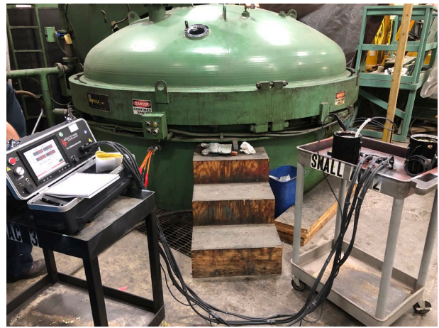
Fig. 1. PD surge tester, VPI tank and two stators being tested in air
