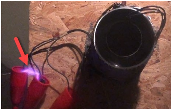
Fig. 9. Arcing at lead connections (purple) due to ionization of remaining gas
