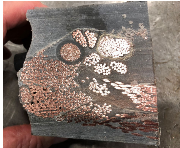
Fig. 10. Vacuum encapsulated stator with voids due to adding material after vacuum encapsulation. Voids progress through stator end with exits by leads.
