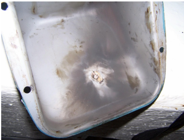
Figure 8: Connection Box Point of Failure
