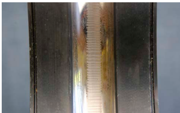
Figure 5-6. Bearing failures due to ASD-induced current flows (fluting). Photo from Electro Static Technology
