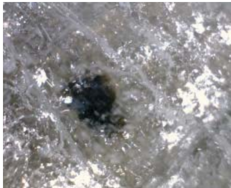
Burned material in insulation layers as magnetic termites gather at a single point.
