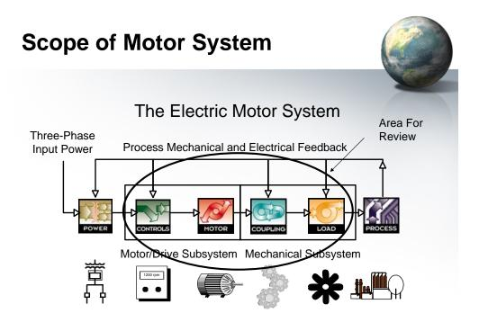
The scope of the analysis will be limited to the MCC bucket through to the Driven load, in this case the pump. Therefore, we will be reviewing the components of the controls, motor, coupling and load, which will also include the cabling between the MCC and motor.
