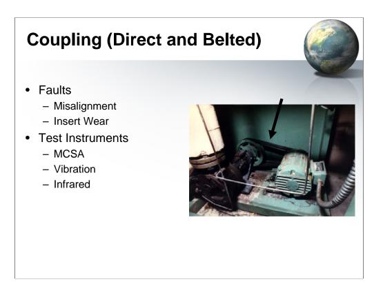
The coupling between the motor and load also has faults due to wear and application:
