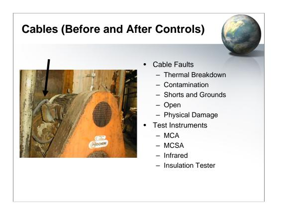
System cabling problems are rarely considered and, as a result, provide some of the biggest headaches. Common cable problems include:
