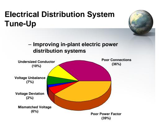
Problems in the system before the electric motor can be broken down in the following order:
