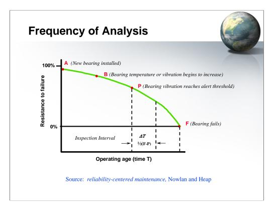
The optimal frequency for testing is based upon the time to failure. With a new component, the resistance to failure is very high, in this case, a bearing. As time continues and the bearing begins to break down, the temperature and vibration increases. At some point before failure, the vibration level will reach some threshold.
