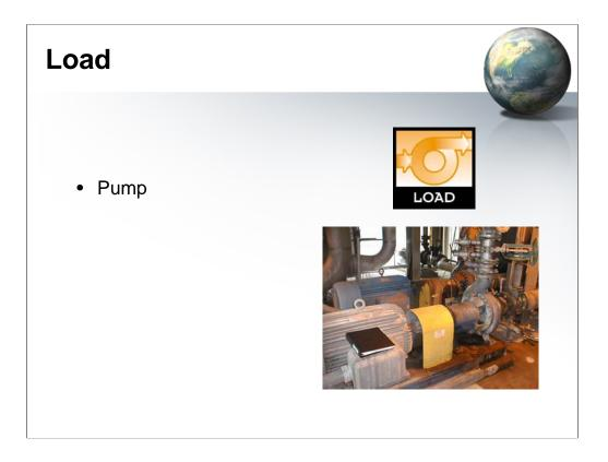
There are a large variety and design of pumps. In this case, we will consider the pump to be of a basic design consisting of a shaft, bearings, mechanical seal, impellor and housing.
