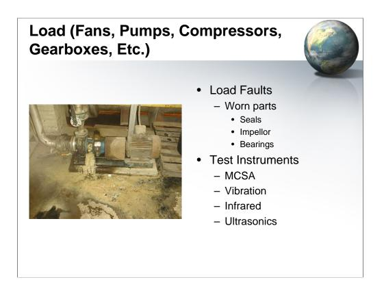
The primary load faults are worn parts such as the seal, bearings and impellor
