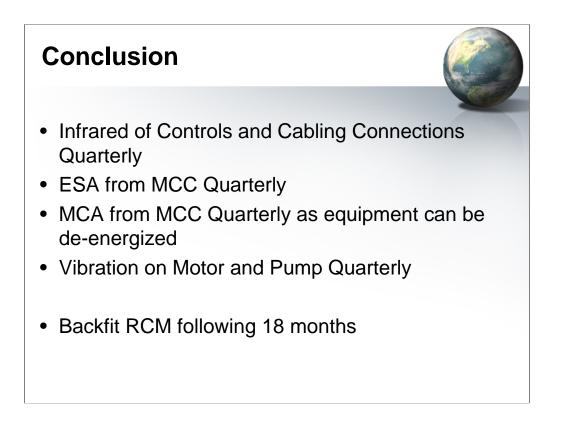
The conclusion from this example would be to perform an infrared inspection of controls and cabling connections quarterly; Perform ESA from the MCC quarterly; MCA from the MCC quarterly, and as equipment can be de-energized; Perform vibration on the motor bearings and pump quarterly. In addition, stagger the tests in such a way to increase the frequency of inspection, should this be a critical or safety related system being tested.
