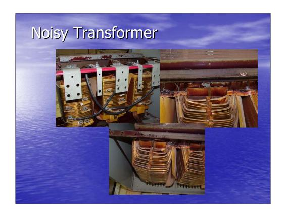
This 150 kVA transformer had been in operation for about 9 years and was becoming noisy. Visual identifiers showed bluing around the top center of the transformer indicating the loose coil. In order to determine if a fault existed, an MCA was performed using the ALL-TEST IV PRO 2000 and following the IEEE 389 test method for transformers.
