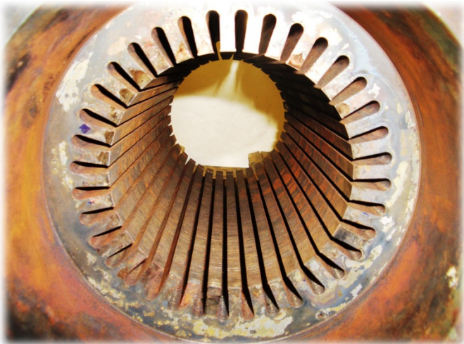
Figure 1: Stator Stripped In Burnout Oven
