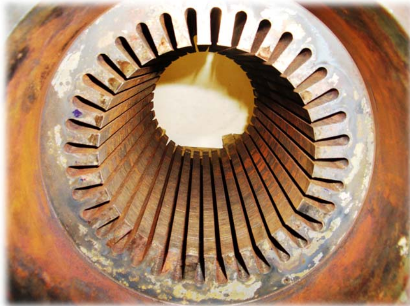
Figure 1: Burned Out Stator Core
