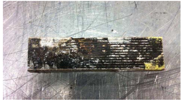
Fig. 3. Inspection of a section of failed coil after tape removal showing surface damage on conductors only indicating ground fault
