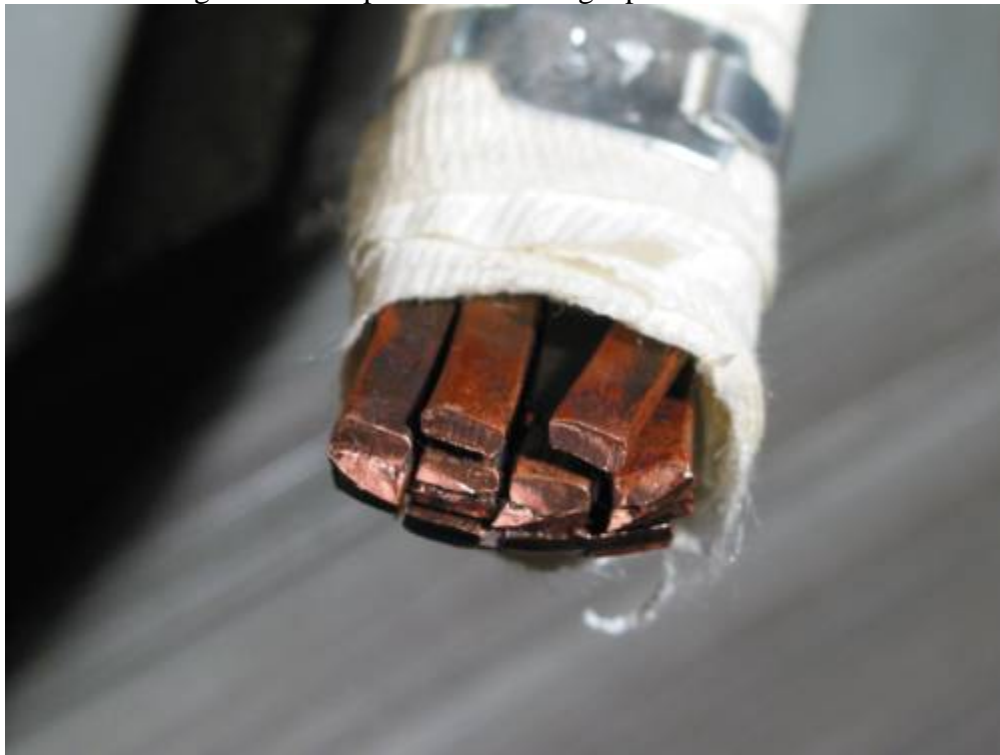
Figure 1: Multiple Wires Making Up One Conductor
