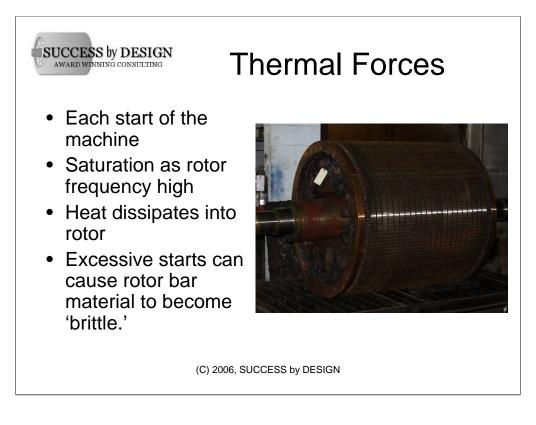
Another key force that acts on the rotor bars is thermal force. This involves the temperature of the rotor bars and rotor iron and the effects of each.
