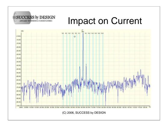
In this example of a 4160 Volt motor with two broken rotor bars, a common rotor bar signature is identified as two distinct peaks plus and minus the pole pass frequency from the supply frequency. Measured in dB, the relative force can be determined, which provides a method of determining the severity.
