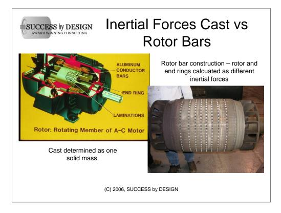
As the induction motor changes speed, including starting and stopping, its circumference and mass resists the change to speed. This is called inertia. You could consider it almost a 'braking' force that is put on the machine as it accelerates or decelerates.
