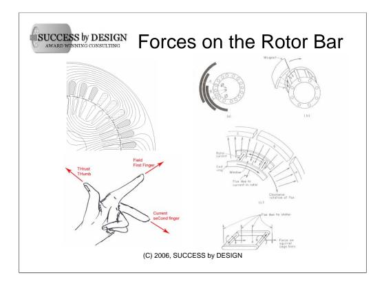
One of the primary forces on the rotor bar is actually indirect. It involves the rotating magnetic fields of the stator crossing the airgap and embracing, or cutting through, the rotor circuit. The common circuit is referred to as a 'squirrel cage' winding as shown on the right side of the slide.
