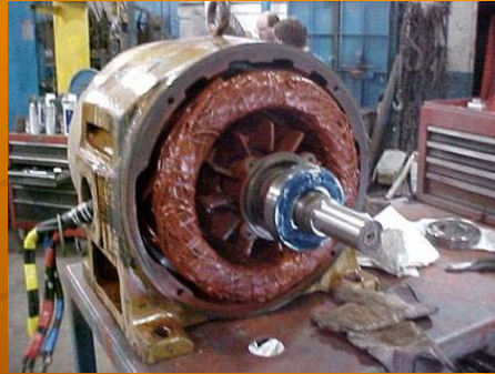
Partially Assembled 125 horsepower Motor in repair shop
