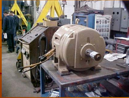
Motor ready for test in motor repair shop
