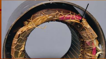
Stage 3 winding failure
