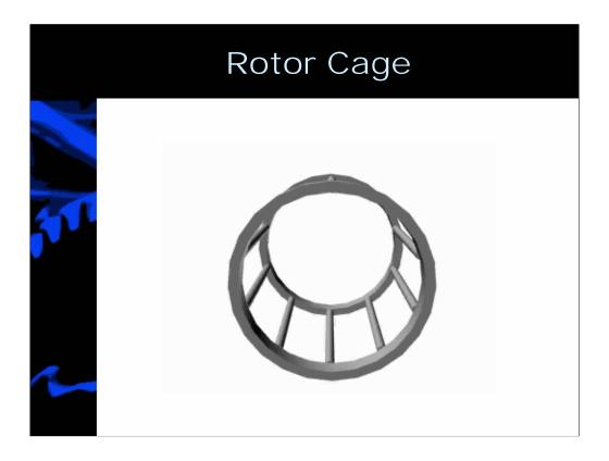
The magnet fields generated from the high current interact with the stator magnetic fields in the airgap between the stator and rotor. As a result, the rotor winding begins to follow the stator rotating field. The rotor can never catch up, however, as the rotating fields must always cut through the rotor bars.
