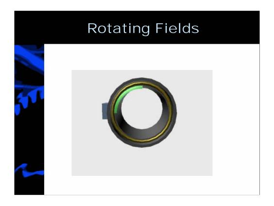
As the three phases of electrical voltage seperated by 120 electrical degrees enter the motor winding, which is seperated by 120 electrical degrees, current and resulting magnetic fields are created. The sinusoidal waveform progressing from a positive value to a negative value generate a rotating field in the airgap of the stator.
