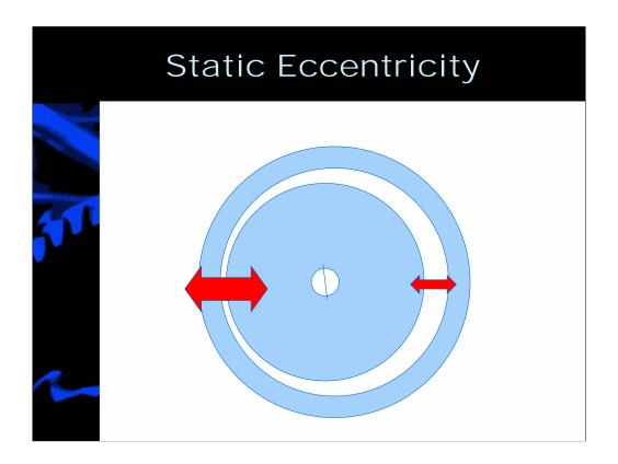
In the case of static eccentricity, where the rotor is operating close to one side of the stator constantly, the magnitude of the interaction of the field on the side close to the stator is higher and away lower. As the north and south fields occur close to the high and low magnitudes, the result is a series of frequency sidebands around the number of rotor bars times the running speed, also known as the rotor bar frequency.
