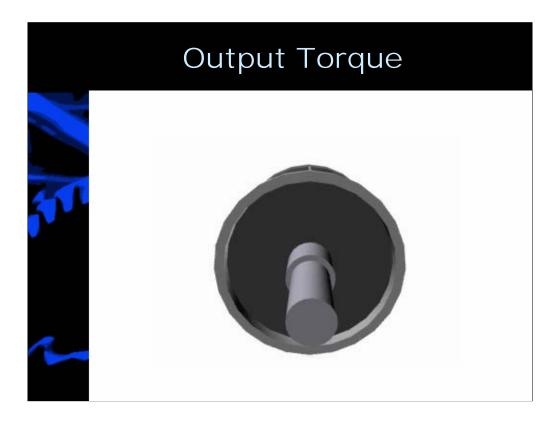
The rotor bars and shorting rings are connected to the rotor shaft, and, as a result, as the squirrel cage turns in the magnetic fields, torque is delivered through the shaft.
