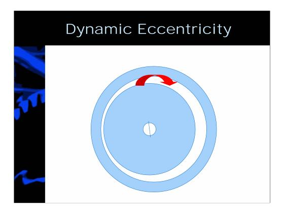
In the case of dynamic eccentricity, the rotor moves within the field at the running speed of the motor. This results in a frequency that is similar to static eccentricity, but with running speed frequencies around the line frequency sidebands.
