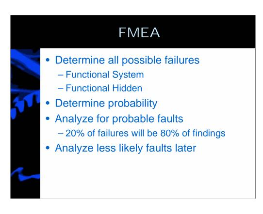
In the Failure Modes and Effects Analysis, the following is performed:
