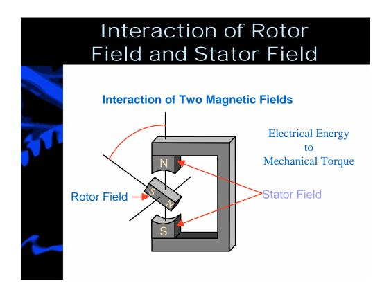
A motor uses the magnetic properties of attraction and repulsion to turn a shaft.
