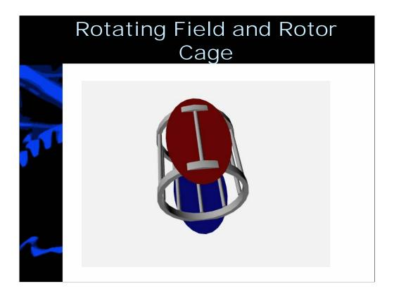
The rotating fields cut through the conductors, or rotor bars, of the rotor. The result is current flow and a second magnetic field. The motor acts, quite literally, as a transformer with a rotating secondary with the stator as the primary and rotor as the secondary.
