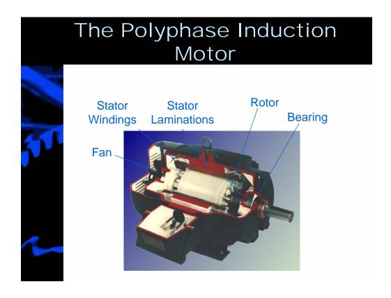
This is a cutaway of a three-phase induction motor.
