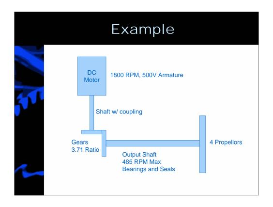
The system under review consists of a DC drive, a DC motor, a shaft with a coupling, a right angle gear with a 3.71 gear ratio, an output shaft that has bearings and mechanical seals and a four blade propellor on the output.
