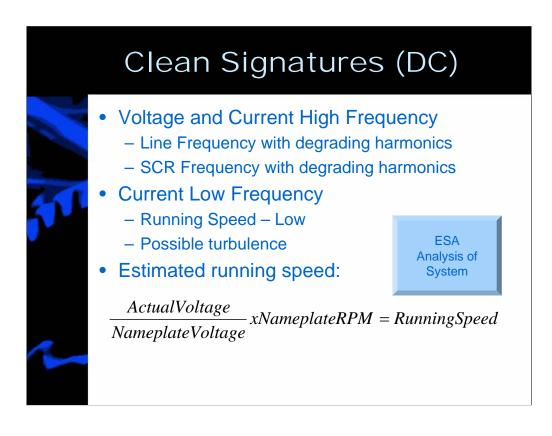
In voltage and current high frequency FFT's, there should be line frequency peaks with degrading harmonics and there should be SCR frequency peaks with degrading harmonics.
