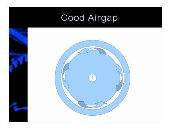
In a perfect motor, the rotor is centered in the stator and all of the fields are even. If a perfect voltage sine wave is introduced, a perfect current sine wave results.
