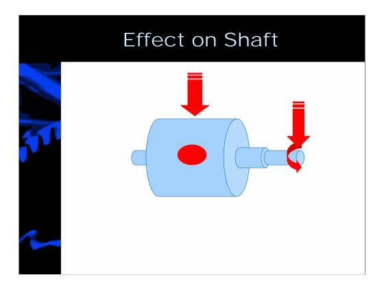
The shaft and rotor in the motor is not truly rigid. It moves.
