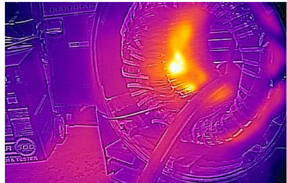
Figure 9: Motor Stator during Hot Spot Core Testing
