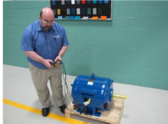
Figure 5: MCA being performed with an ALL-TEST Pro 5 on a completed motor
