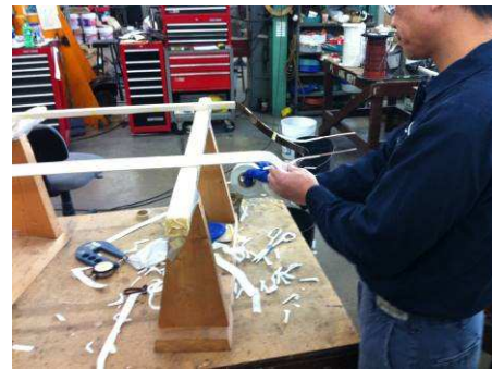
Fig. 6. Armor Tape on Formed Coil
