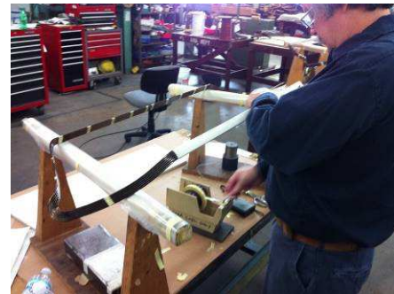
Fig. 5. Wrap Filler in Slot to Ensure the Coil is Tight in Slot
