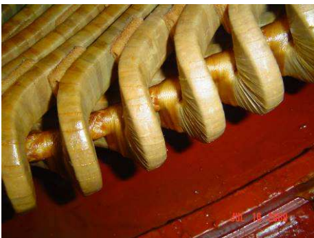
Fig. 9. Surge rope, blocking and ties on a VPI processed winding
