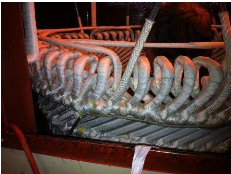
Fig. 8. Surge rope and ties on a green winding
