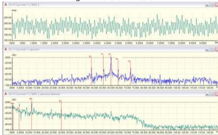
Figure 9: Fan and Belt Faults
